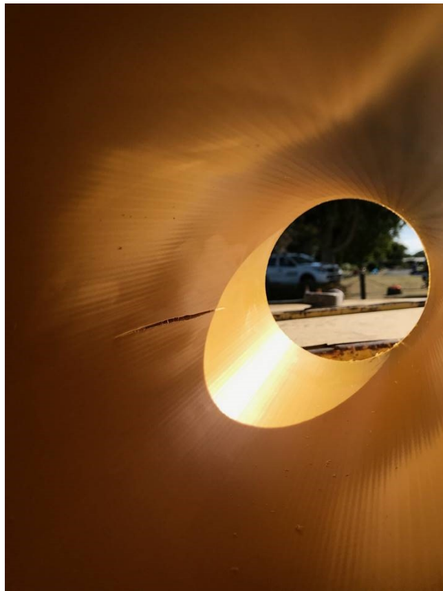
Figure 6.7: Photo of longitudinal cracking on Pre85 sample
