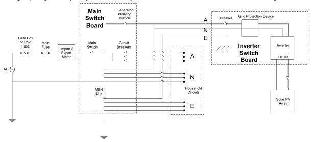
A UPS type system with appliances connected between the inverter and the grid protection device. Note the red lines showing the inverter circuit. In a UPS circuit, no residual current devices shall be placed between the point of supply and the inverter. The same is true for any protection device that breaks the neutral conductor.
